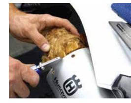
You can see that the bottom of the core on the FE muffler is all banged up. Seems like a lot of them are that way from bad assembly practices. You may have to grab the pliers and straighten it out or make it round again before you install the new end cap.
