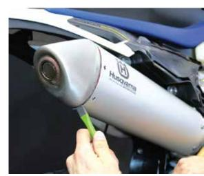
When the end cap comes off, there is some packing material that sticks out of the end. You will want to remove it by cutting it off. It cuts off pretty easy with a sharp razor blade. Cut so that it's about flush with the end of the muffler can.
