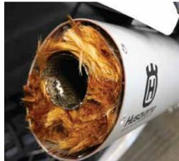
Tap the new end cap in. It goes in a lot easier than the old one came out. You can see here how far off the can's screw holes are.
