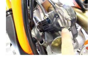
Go ahead and take the fuel line off of the old fuel and place on the new rail with the new hose clamp. Put a little lube on the injectors red O ring and slide into the fuel rail.
