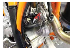
Put some grease inside the rubber air boot, where it fits over the throttle body and make sure the clamp is nice and loose. This will help it fit back over the throttle body easily, when you lower the sub frame back down. Wiggle the body around a bit if needed to help it fit back in. Now tighten it all back together.
