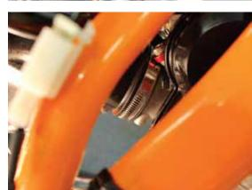
The longer piece of fuel line that is provided goes here between the tanks fitting and quick disconnect, if needed. If you are using our 90 degree tank fitting, you can use this and cut to size or use the stock line. This picture is missing a hose clamp on one side, but don't forget it!
