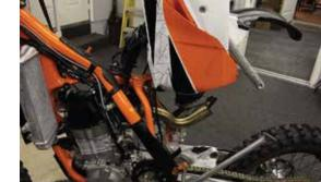
Once up, tighten down one of the upper subframe bolts and it should stay up and out of the way. Now you can easily get yo your fuel rail.
