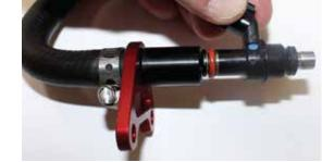
You can now install the injector assy back into the throttle body and secure with the new, supplied allen screws.
