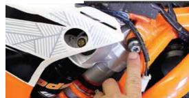
3. Remove the lower 2 subframe bolts and just loosen the top 2 subrame bolts, do not remove them.
