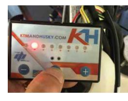
The final notes on tuning with this programmer is, when in the Green, Yellow or Red modes, which are modes 1,2 and 3. Pushing the plus button and raising the number of where the light is flashing, adds fuel. And pushing the minus button takes fuel away.
