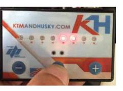
Now push the "mode" button again and it takes you to the red lights. You will want to push the "plus" button until lights 5 and 6 are both lit up. When you move the lights to the right, with the plus button, you add more fuel. This will set the air/fuel ratio perfectly, for when you have the throttle wide open and the bike get's into the high rpm's.
