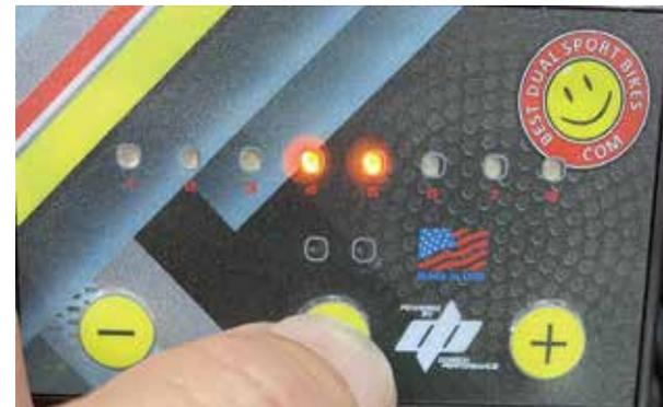
The 3rd mode, RED lights, you will want to set to the number 3 position (one light). This will provide an AIR/FUEL ratio of 12.5:1 when the bike is running above 7500 RPMs. This is true whether you are running an open exhaust or using our end cap. It runs in the same area with the stock header or De-cat header and stock airbox lid or more of an open lid.
