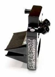
The rest of the procedure is pretty easy. The injectors fit into the new block as so. You can grease the o rings on the injectors if you want. The top plate fits on and screws to the main plate with the 2 smaller allen head screws in the kit.
