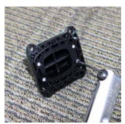
Remove the 4 small torx head screws that hold the 2 parts of the reed block together.
