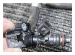
If you expand and pull on the metal clip, then it will release the injector and you can pull it out of the stock fuel rail.
