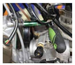
Now loosen the clamp that holds the throttle body in the rubber boot and pull it out. Remove the 4 8mm head bolts that hold the reed assembly to the crankcase and pull the rubber boot and reeds out.
