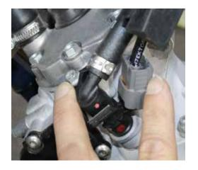
Remove the injector from each side. They are held down by a 8mm head bolt. Pull and wiggle and they will come out.
